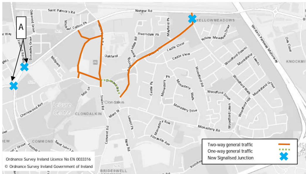
Figure 5.27: Route Option S2-4 – Clondalkin Village Proposed General Traffic Strategy (Principal Local Road Access Network affected by CBC)
